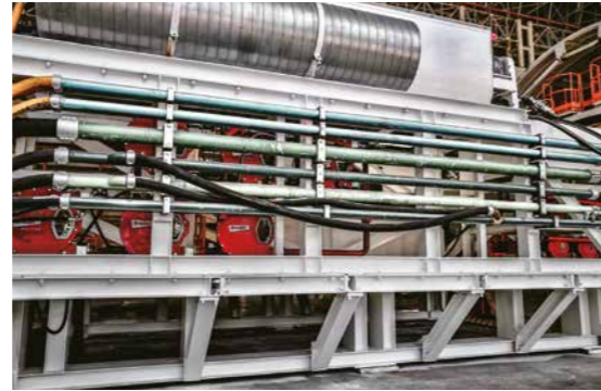
▲ Breidel pumps used for grout and accelerator pumping for solidification of concrete rings
