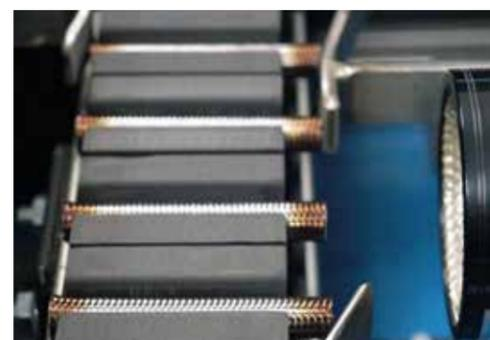
In addition, Aflex has developed a fully automated inspection system which verifies the internal bores, braid outer diameter, flare diameter and hose length, ensuring only products that are 100% fit for purpose are sent to the customer. This inspection system is only applicable to regularly supplied large quantities of cut lengths and is limited to cut length which are less than 150mm (5.9 inches) in length.
