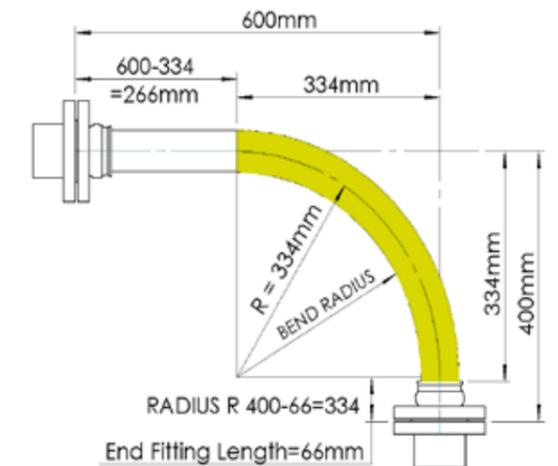
Note: The bend radius is measured to the inside edge of the hose, For the minimum bend radius please refer to page 8.
