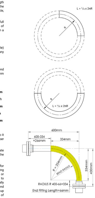
Note: The bend radius is measured to the inside edge of the hose, For the minimum bend radius refer to page 6.
