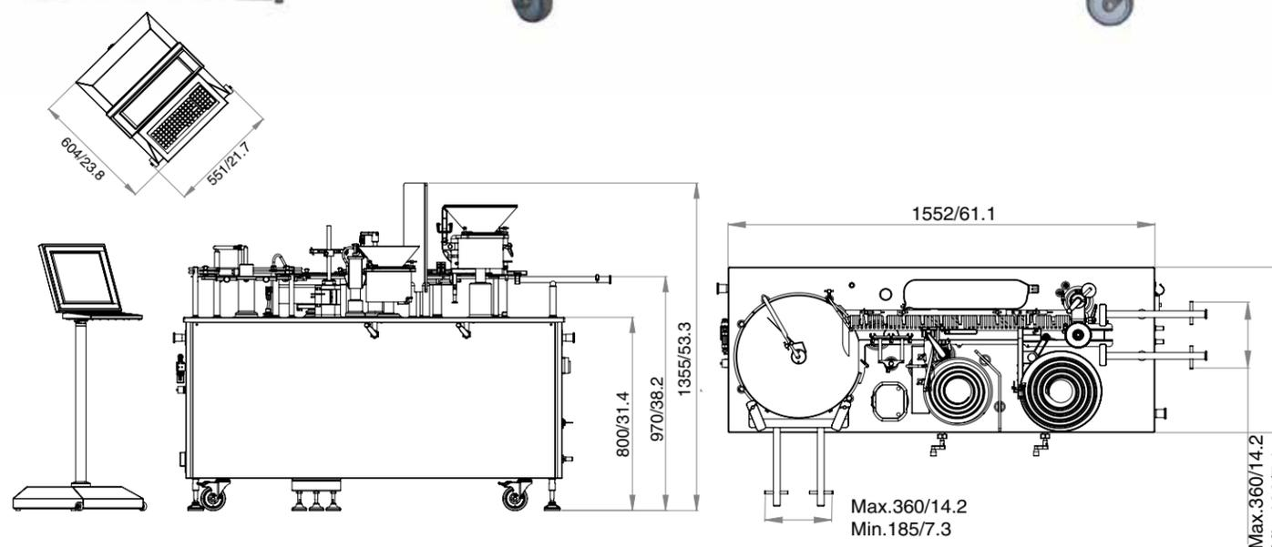
All dimensions in mm/inch. This drawing includes optional inline check weighing. The infeed tray can be mounted on the left side or on the front of the machine and the FPC50 can be customized for integration into RABS or isolators
