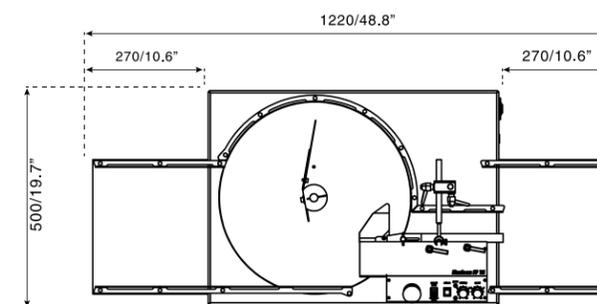
Dimensions in mm/inch. On FlexFeed20 and FlexFeed15 the infeed tray can easily be mounted on the front or on the left side of the machine.
