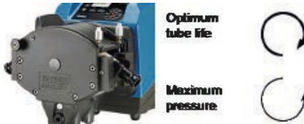
Figure 3 - Rotor direction
