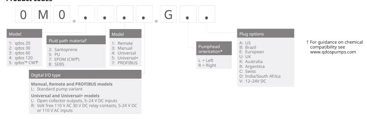
\* The pumphead side location is required when ordering. The left/right perspective assumes the user is looking at the front of the pump. The pump in the dimensions diagram is considered a pumphead located to the left.
